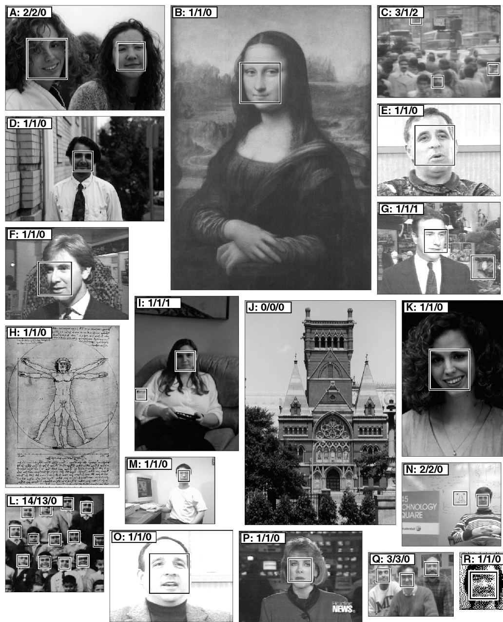
Fig. 13. Output obtained in the same manner as the examples in Fig. 11. Some notes on specific images: Faces are missed in C (due to blurriness) and L (due to partial occlusion of the chin). False detections are present in C, G, and I. Although the system was trained only on real faces, hand drawn faces are detected in H and N. A, D, I, J, and K were scanned from photographs; B, H, and L were obtained from the World Wide Web; C, E, F, G, O, and P are digitized television images. M, N, and Q were provided by Sung and Poggio at MIT, and R is a dithered CCD image.
