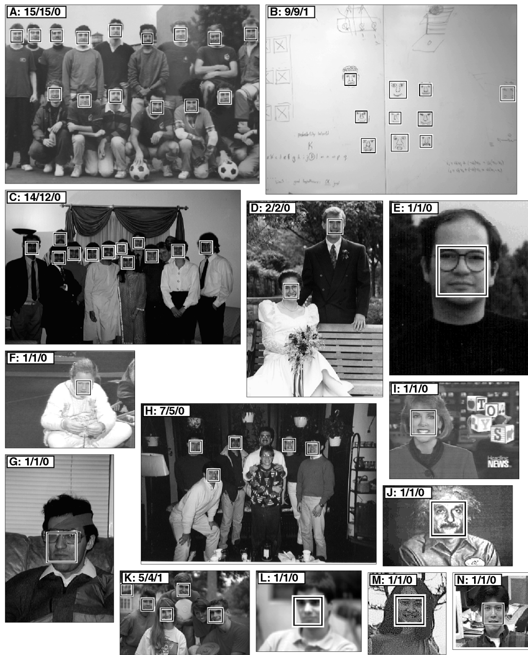
Fig. 12. Output obtained in the same manner as the examples in Fig. 11. Some notes on specific images: Faces are missed in C (one due to occlusion, one due to large angle), H (reflections off of glasses made the eyes appear brighter than the rest of the face), and K (due to large angle). False detections are present in B and K. Although the system was trained only on real faces, hand drawn faces are detected in B. A, B, J, K, and L were provided by Sung and Poggio at MIT; C, D, E, G, H, and M were scanned from photographs; F and I are digitized television images; and N is a CCD image.
